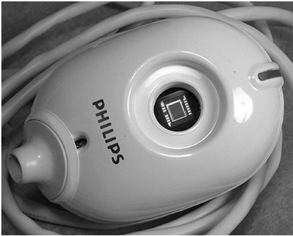
FIGURE 51. CCD image sensor (in webcam with lens removed)
